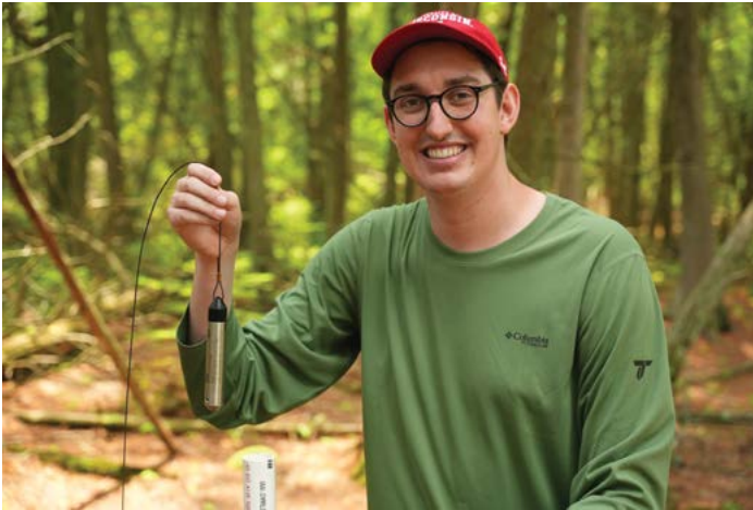
Kastelic collects a pressure transducer that regularly measures groundwater levels under forested ridges.
