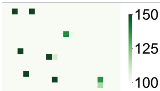
Raman map of 1.5 µm microplastics. Raman mapping can identify and visualise microplastics/nanoplastics down to 100 nm.
