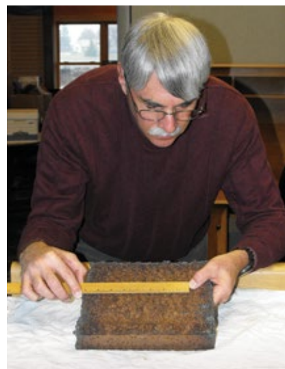
Clark measuring corrosion pit sizes in a steel "coupon" that was placed in the Duluth harbor as part of his work on freshwater steel corrosion.
